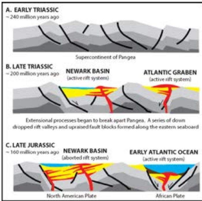
**Figure 4.** Diagram showing a simplified timeline of the formation of the Newark Basin. *Modified from U.S. Geological Survey, 2015*
