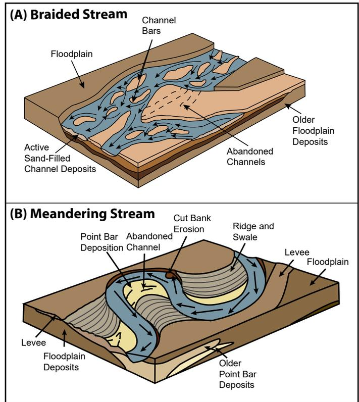
**Figure 7.** Diagram showing the river channel of a braided river system and meandering river system. *Modified from Schieber, 2007*
